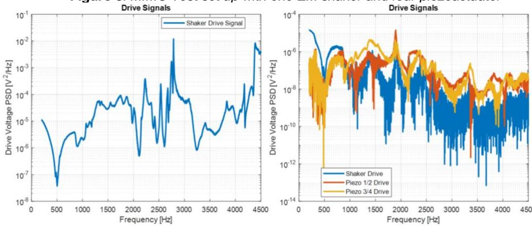
**Figure 4:** (Left) Shaker drive voltage, (Right) MIMO drive signals for the HDD case
