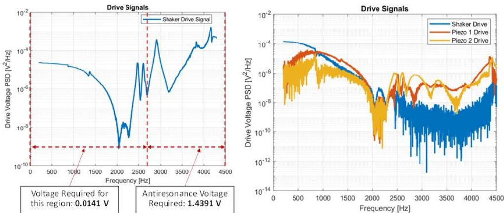
**Figure 2:** (Left) Shaker drive showing antiresonance voltages, (Right) MIMO drive for dual piezo case
