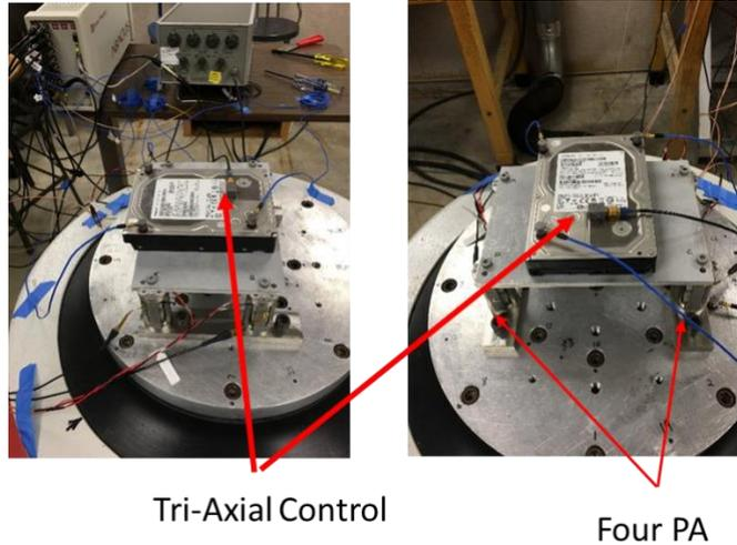
**Figure 3:** MIMO Test set up with one EM shaker and four piezoactuator
