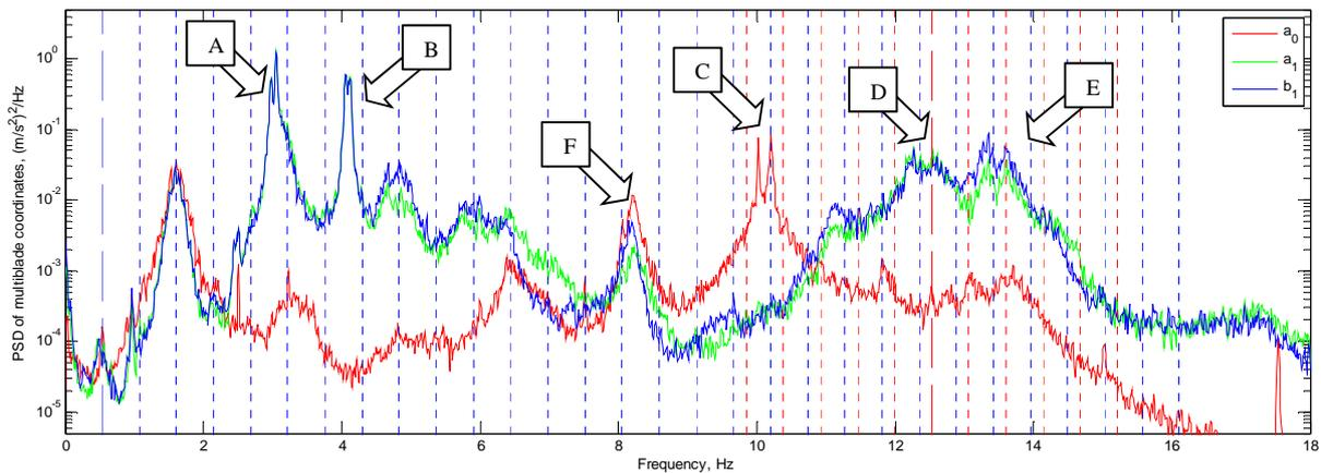
Figure 5 PSD of multiblade coordinates for 3e sensor location.
