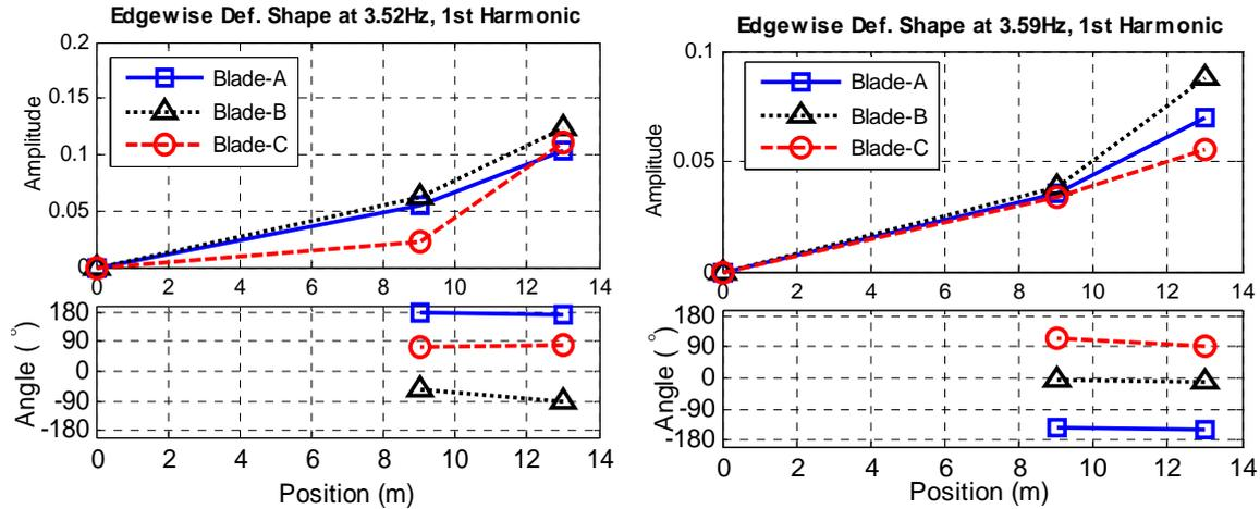
Figure 13 Deformation shape identified by AMI in 1<sup>st</sup> harmonic for modes centered at a) at 3.518Hz b) at 3.587Hz.
