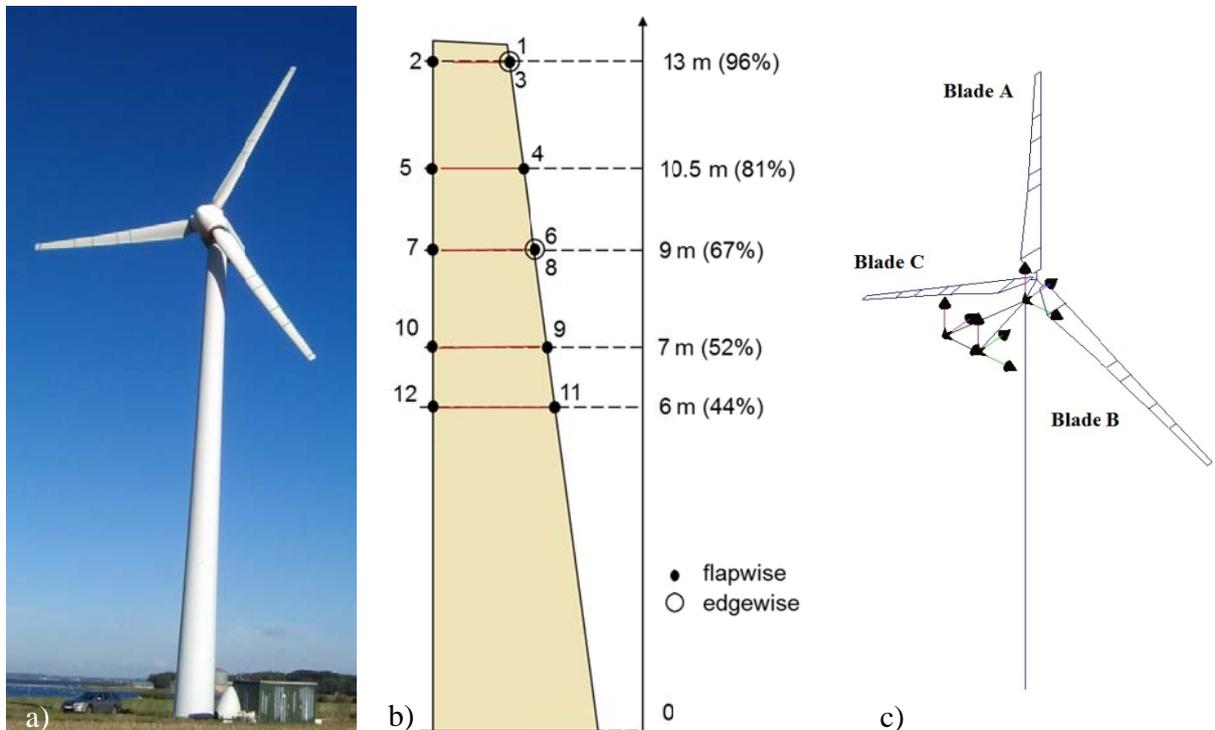
Figure 1. a) Vestas V27 with blades instrumented with accelerometers; b) Location and orientation of the accelerometers on the blades c) Location of triaxial accelerometers in the nacelle.
