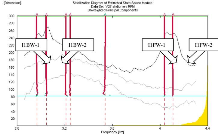
Figure 8 Stabilization diagram around first in-plane modes
