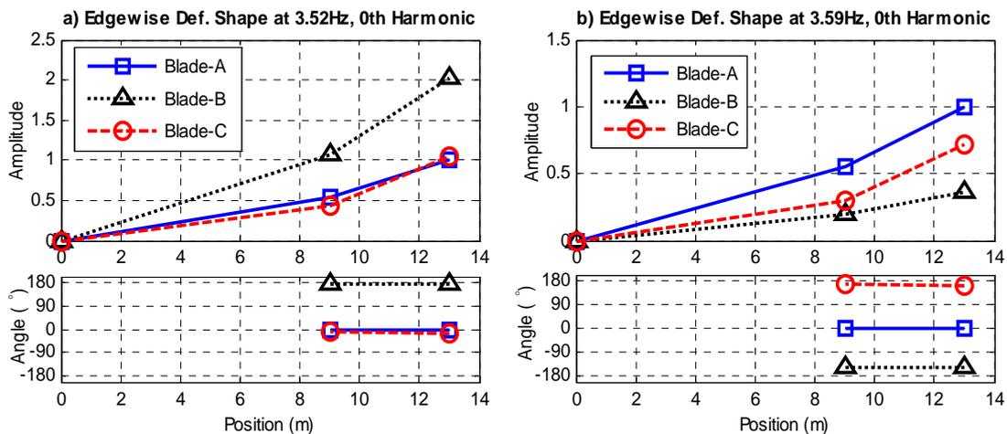
Figure 12 Deformation shape identified by AMI in 0<sup>th</sup> harmonic a) at 3.518Hz b) at 3.587Hz.
