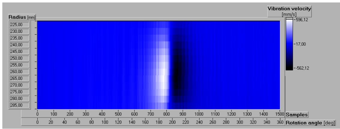
Figure 9: TLDV map on a tyre sidewall
