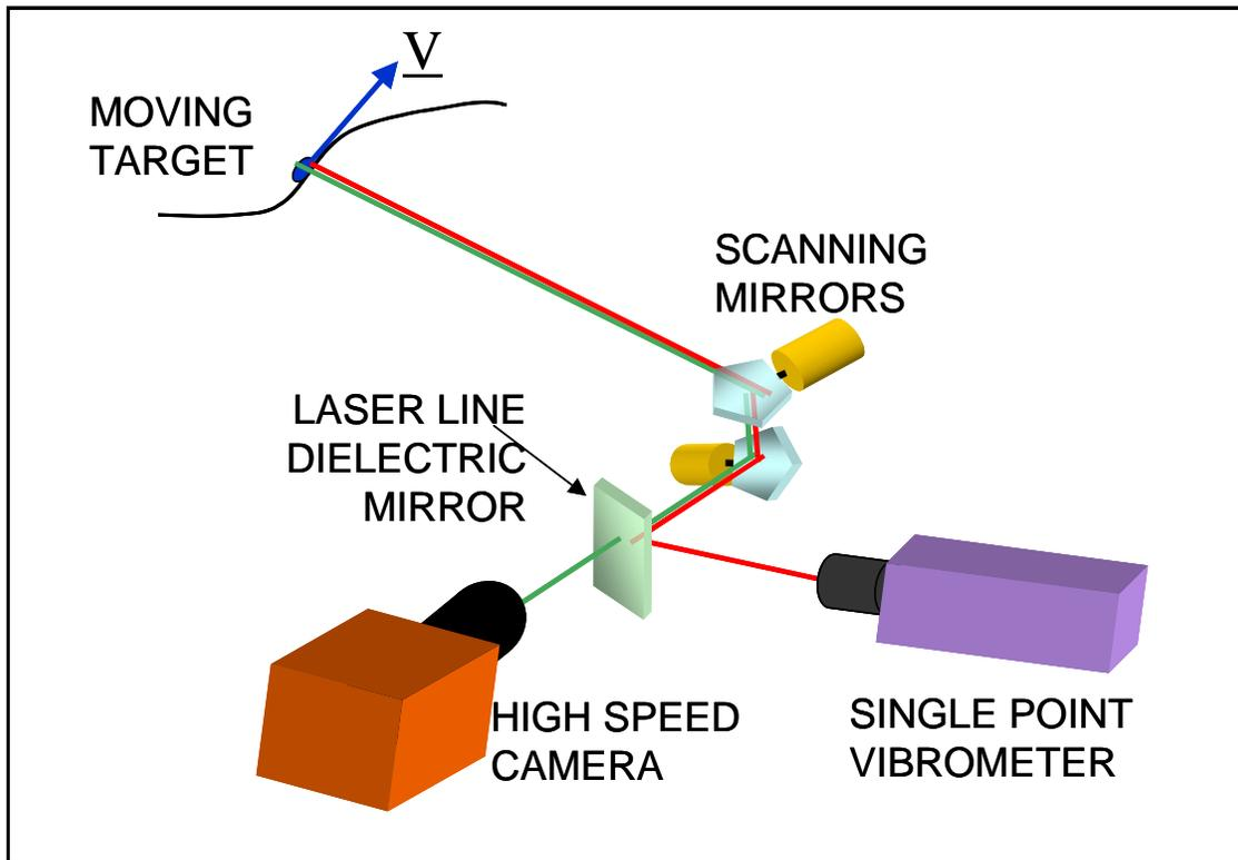
Figure 10: Layout of image Tracking LDV
