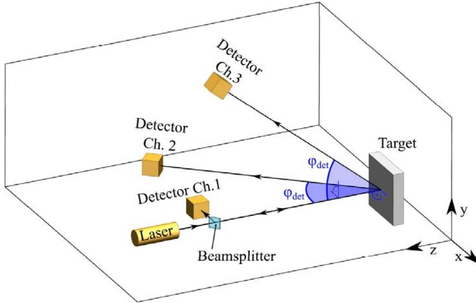
Figure 15: Optical setup for 3D microscope based LDV
