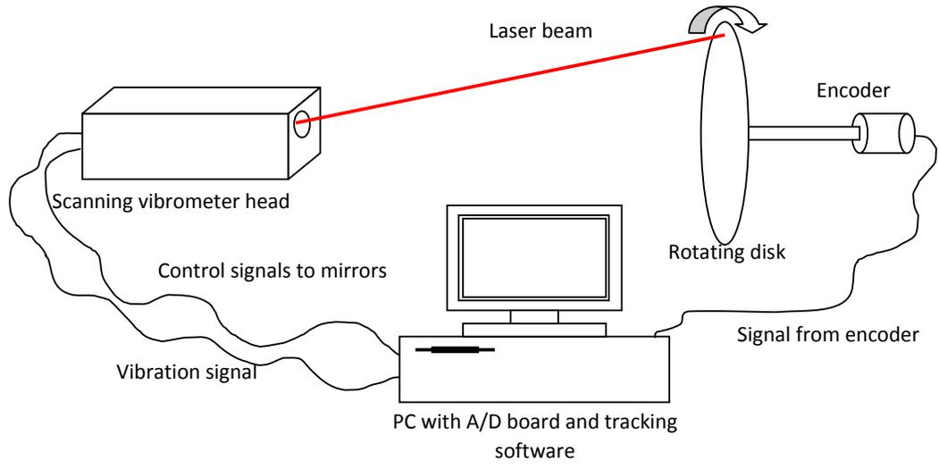
Figure 8: Schematic diagram of the first TLDV system
