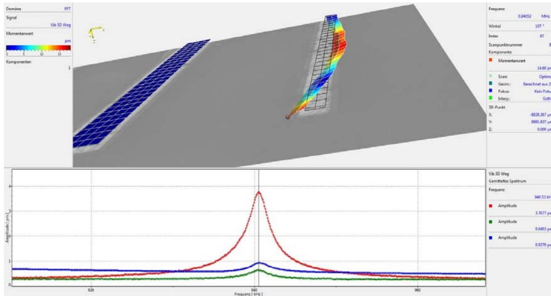
Figure 16: 3D displacement of PZT MEMS cantilever in higher order bending mode
