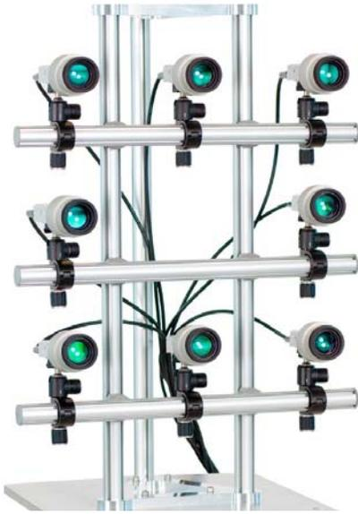
Figure 17: 8 channel optical setup of Polytec Multipoint Vibrometer
