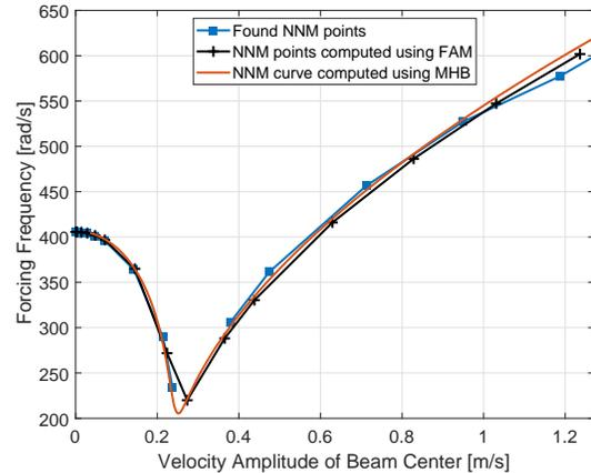
**Fig. 3:** Comparison of the NNM curve computed with the presented algorithm with solutions obtained using the Force Appropriation and Multi-Harmonic Balance Methods
