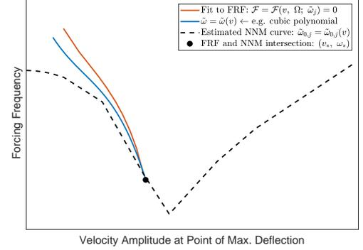
**Fig. 1:** Plot of interpolated frequency response function, effective NNM frequency  $\tilde{\omega}_j(v)$  and estimated NNM curve  $\tilde{\omega}_{0,j}(v)$ . Those three curves would cross one another at point  $(v_*, \omega_*)$  marked with a  $\bullet$
