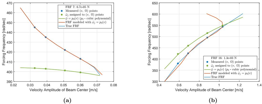
**Fig. 2:** Results of the first two algorithm stages for force magnitudes of (a) 6.7e-5 N (the system exhibits softening at this force level) and (b) 1.3e-3 N (hardening)
